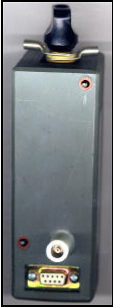
Fig. 6 : Plug-On Shunt with Triaxial Plug
